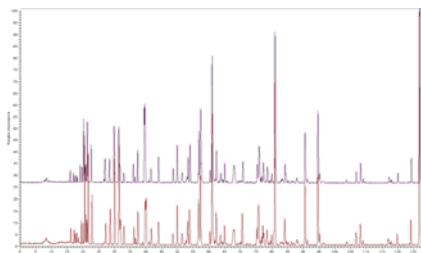
Figure 1. Reproducibility for a 3-35%B gradient in 80 min of a BSA tryptic digest on a 80 cm column. Maximum backpressure was 9,800 psi
